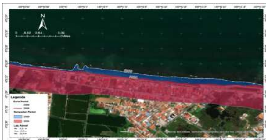
Figure 1.1. GIS Data on Coastal Line Shifts Inland from 2009 to 2024
